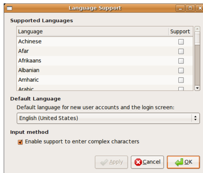
Figure 3. The “Language Support” window. Make sure the “complex characters” checkbox is checked.
